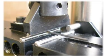
3-point bend testing
